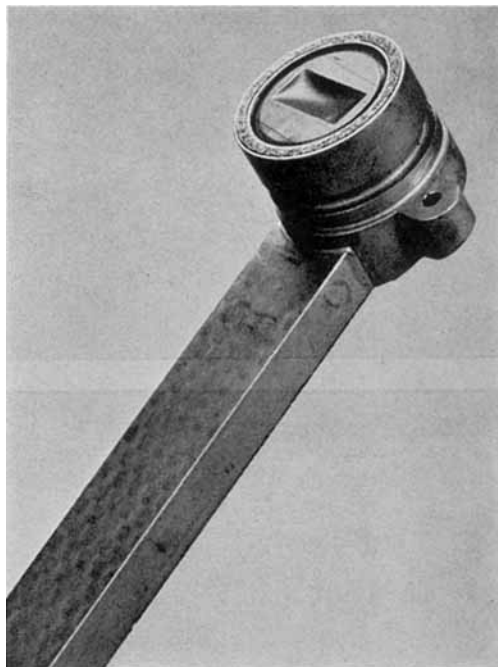
Fig. 5. Teflon window across feed end of the microwave antenna of a guided missile (courtesy of the Microwave Journal ).
